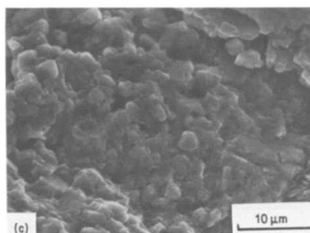
5. The pretreatment in N<sub>2</sub> atmosphere was found to accelerate the grain growth of diamond in both unary and binary solvent-catalyst systems.
