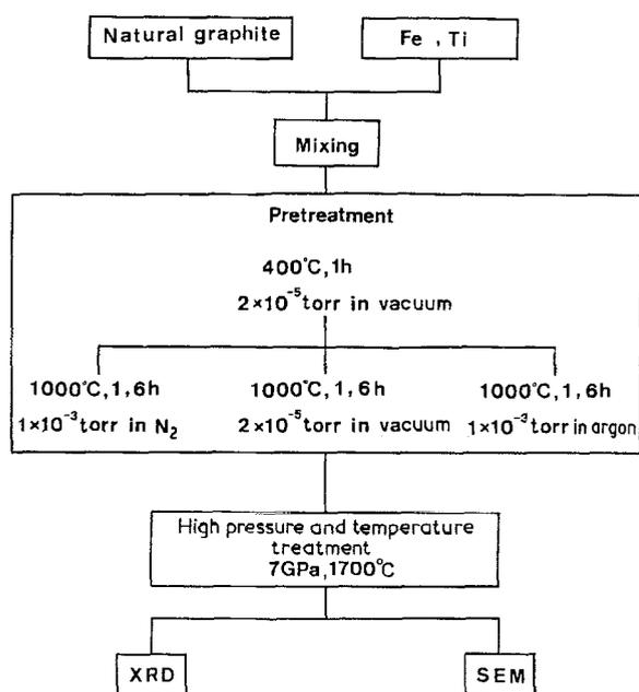
Figure 1 Experimental procedure for conversion from graphite to diamond.
