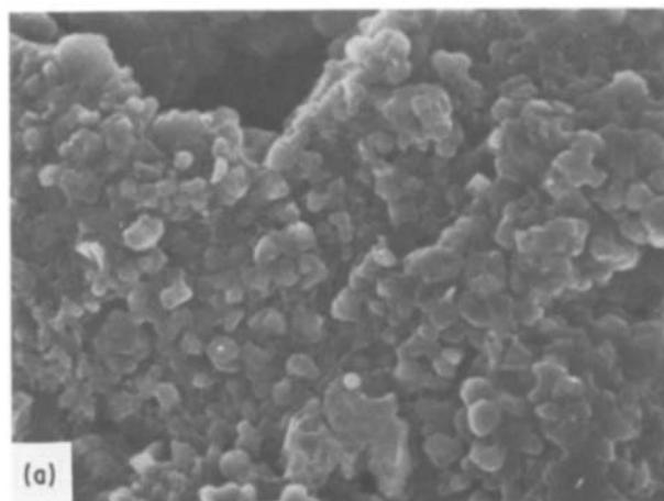
*Figure 5* SEM photographs of the fractured surface of diamond treated at 7 GPa and 1700°C for 1 min in the presence of 10 wt % Fe-10 wt % Ti after the pretreatment at 1000°C for 1 h; (a) in vacuum, (b) in argon and (c) in N<sub>2</sub>.
