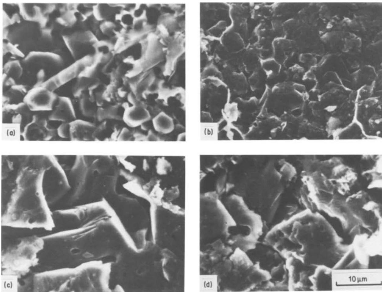
Figure 3 SEM photographs of the fractured surface of diamond treated at 7 GPa and 1700°C for 15 min in the presence of 10 wt % Fe-10 wt % Ti after the pretreatment at 1000°C for 1 h; (a) in vacuum ( $2 \times 10^{-5}$  torr), (b) in argon ( $1 \times 10^{-3}$  torr), (c) in  $N_2$  ( $1 \times 10^{-3}$  torr) and (d) with no pretreatment.
