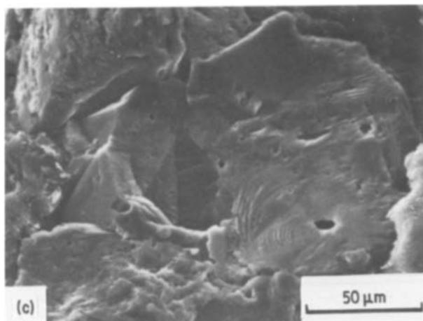
*Figure 4* SEM photographs of the fractured surface of diamond treated at 7 GPa and 1700°C for 15 min in the presence of 10 wt % Fe-10 wt % Ti after the pretreatment at 1000°C for 6 h; (a) in vacuum, (b) in argon and (c) in N<sub>2</sub>.
