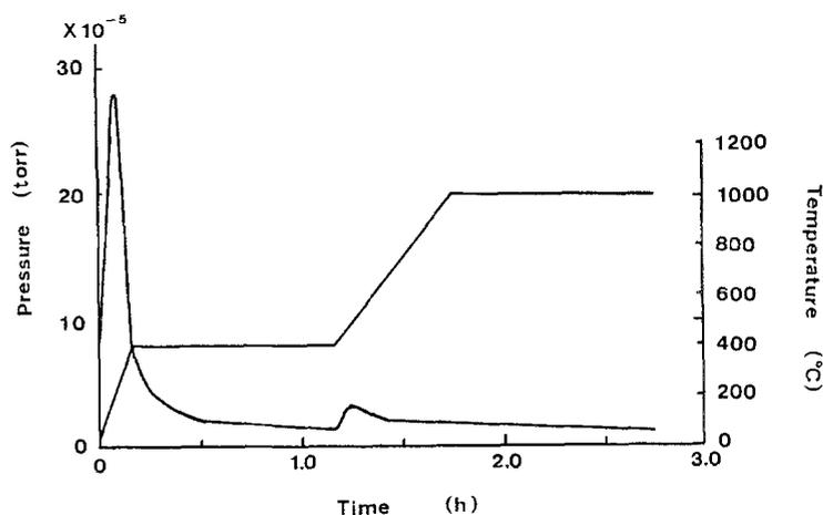
Figure 2 Pressure and temperature variation in the furnace as a function of pretreatment time.
